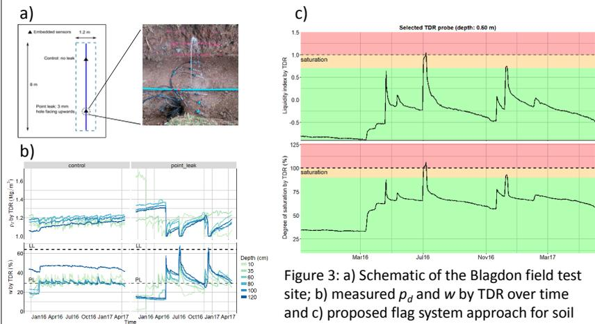
Figure 3: a) Schematic of the Blagdon field test site; b) measured  $\rho_d$  and  $w$  by TDR over time and c) proposed flag system approach for soil condition monitoring with TDR.
