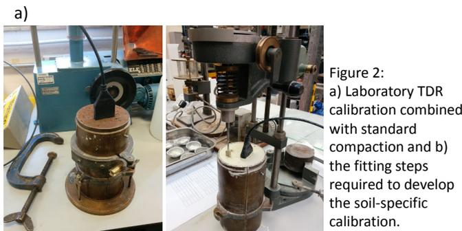
Figure 2: a) Laboratory TDR calibration combined with standard compaction and b) the fitting steps required to develop the soil-specific calibration.
