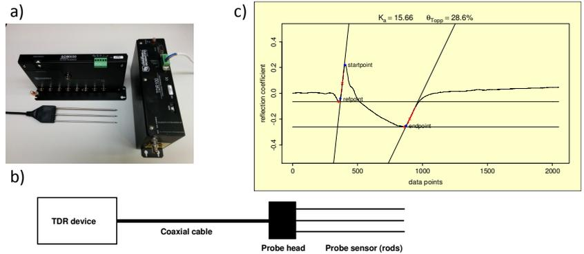
Figure 1: a) the TDR unit, multiplexer and 3-rod probe used in this study; b) schematic of the TDR system without multiplexers and c) example of TDR waveform analysis in soil.
