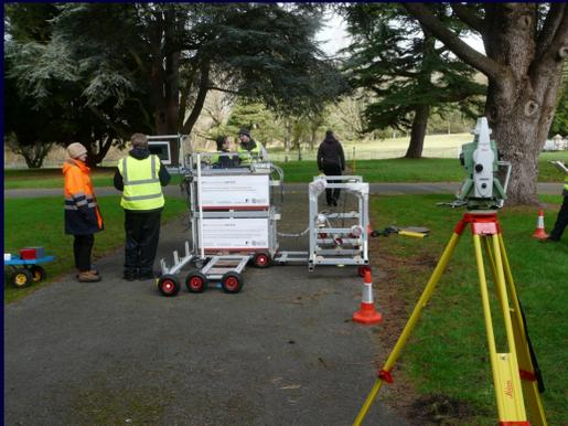
The only significant mutual interference problem encountered was with the magnetic detection. The coils needed to be more than 0.7m from the rest of the Mobile Laboratory.
