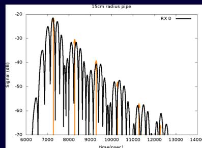
Results from the Bath sandpit with the SFCW radar indicated a relative permittivity of 6.2, while examination of b-scans from a commercial GPR suggested a relative permittivity of about 6. Similarly tests at Wigan produced a relative permittivity of 7.4 with the SFCW radar and 8 from the commercial GPR.
